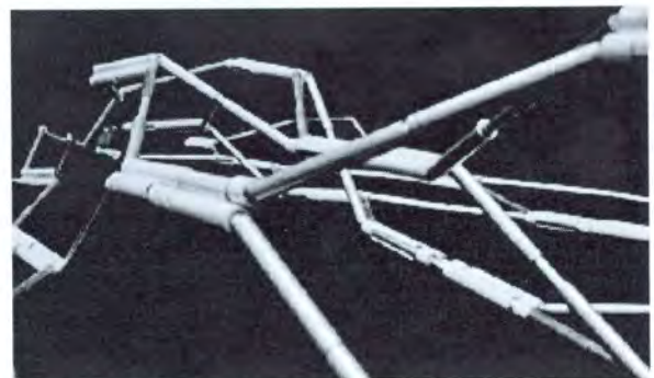
Photo 4 A physical prototype was built by aluminium tubes and PVC to test the actual behaviour of the kinetic tectonic system.
